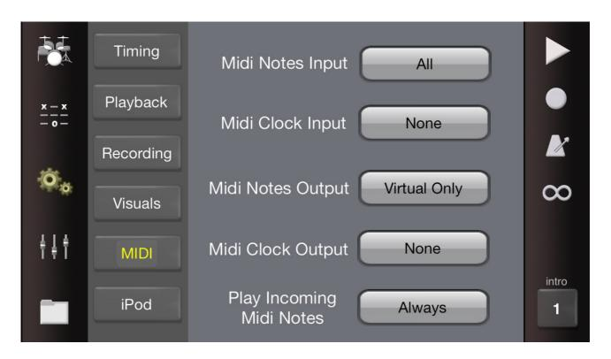
MIDI enables Drumstudio to be played with a physical e-drum drum kit for convenient recording and playback. The iPad version supports external USB Midi controllers via the Camera Connection Kit. To record on the iPhone version you will need an external Midi adapter like the iRig Midi.
